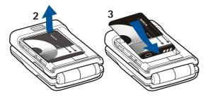
3. Direct the locking catches in the battery cover towards the locking catches on the phone and slide the battery cover into place (4).
